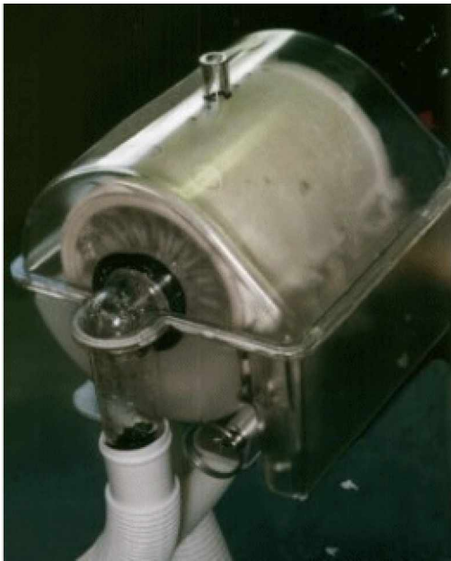
Figure 2, Disposable Rotary Drum Filter in Operation
