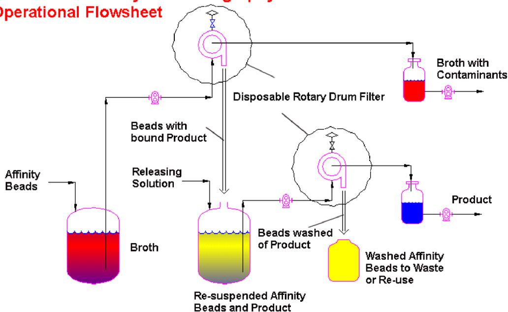
**Note:** If contaminants are initially bound to beads, filtrate from first solid / liquid separation becomes product. Second solid / liquid separation is only needed to recover beads.
