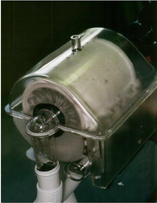
The Disposable Rotary Drum Filter is based on the principles of large scale rotary vacuum filters that have been in operation in various CPI's for years. The challenge in developing this device was making it small enough to accommodate the normally smaller volumes and thus flow rates that would be present in a continuous chromatography system of this type.
